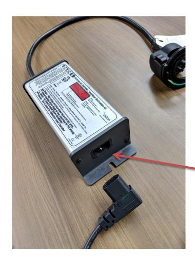
Hold down the button on the side while plugging the power back in.
